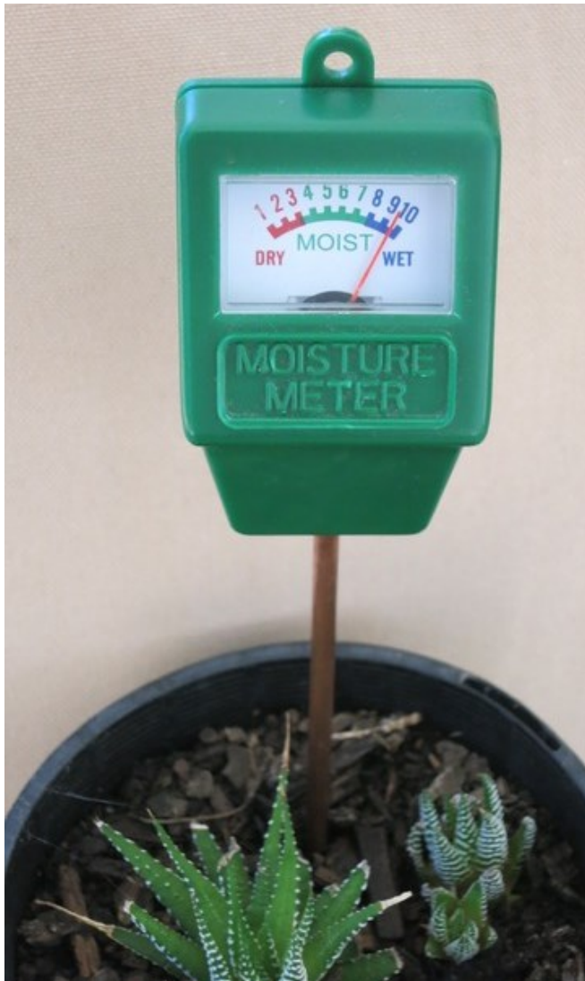
The moisture meter in action (leaving it in the pot is not recommended)
