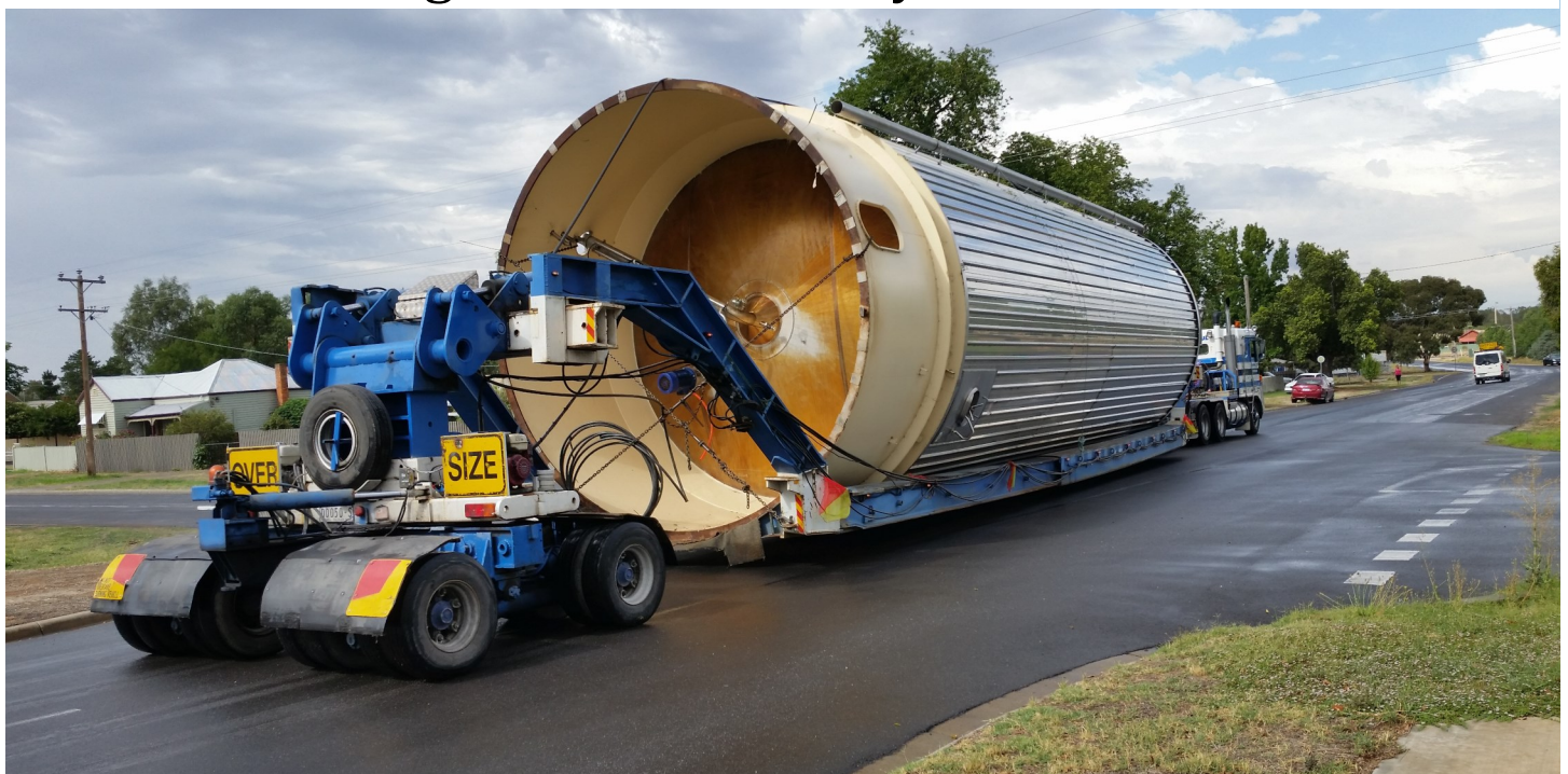
This photograph, taken by Monika Thumerer, is of a enormous silo or tank (or something) being transported through the streets of Dunolly. The vehicle has special turning equipment front and back of the silo, so that the driver can manipulate the turn into tight corners with ease. If anyone knows what this is — please email us on welcomerecords@iinet.net.au
